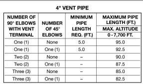
For the 3" and 4" vent, one 90° elbow is equivalent to 5 feet of pipe. One 45° elbow is equivalent to 2.5 feet of pipe.
